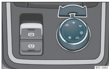
Fig. 146 Console centrale : Commande rotative (Driving Experience button).
